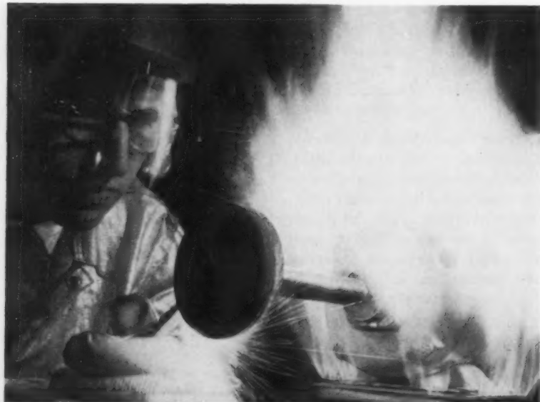
HOT WORK: Despite intense heat from jets of burning gas, this experimental Westinghouse Electric Corp. motor still operates well enough to do this grinding job. Special insulation makes it possible.
